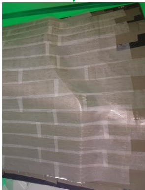
Adhesive and GF layers patched directly on core
