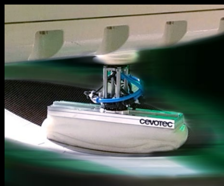
Form-flexible patch grippers support the automated and precise fiber lay-up for monolithic and sandwich components.
