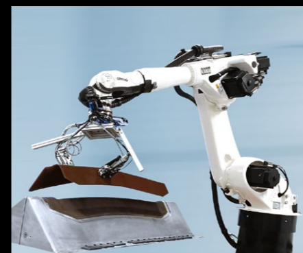
Robotic honeycomb placement precisely places 3D core material directly on the laminate with a dedicated gripper.
