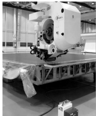
Automated Tape Laying
