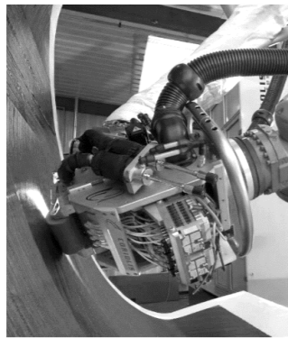
Automated Fiber Placement
